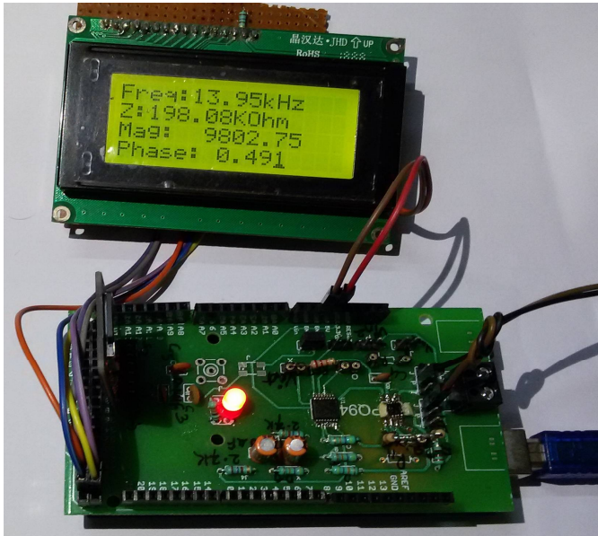
Fig 4 : impedance analyzer system based on AD5933
